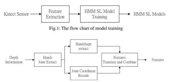
Fig.2: The detail flow chart of feature extraction
